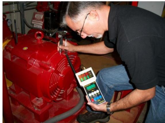
**Figure 3: Vibration analysis tool indicator**
