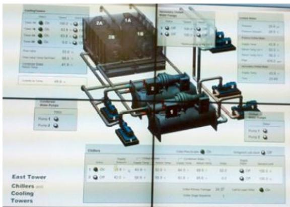
Figure 7: IBIS view of chilled water plant
