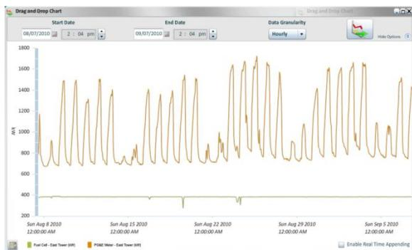
**Figure 8: Trend data comparing energy consumption from the utility to energy generated by fuel cells in the East tower**
