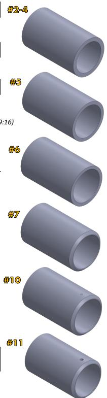
12) Countersink all three Ø.150" holes – indexing 120 degrees each time. Cut approx. .010" deeper to account for clean-up cut on OD in final step. Set quill stop or Z axis digital readout for consistent depth. (16:45)
