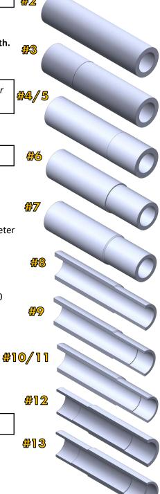
14) Cut .05" X 45° internal chamfer. (28:40)
