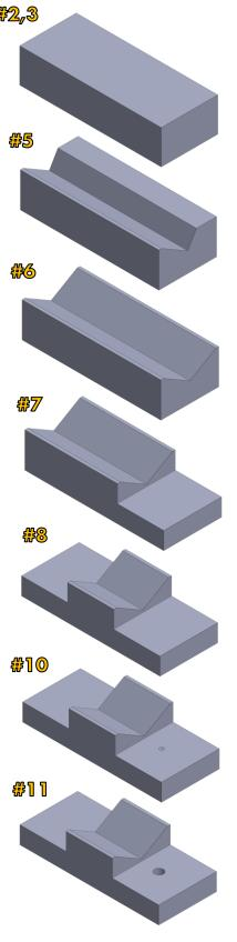
6) Mill other vee surface using scribed lines as reference. Verify depth of vee by measuring from bottom of part to top of Ø.750" gage pin (should be 1.23"). (19:40) Tools used: 1/2" HSS end mill, digital readout
