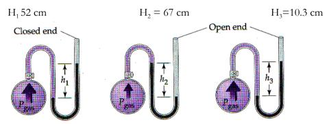
In a closed end manometer, the pressure exert is the height of the column of mercury, the P is 520 mmHg. The problem, though, is asking about the open end manometers. In the second manometer, the atmospheric pressure is exerting a force on the gas. The pressure of the gas is
